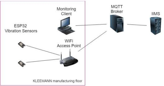
Figure 5 - UC-KLE-1 Sensors Network Architecture
