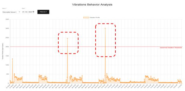
Figure 25 - Abnormal Vibration Threshold
