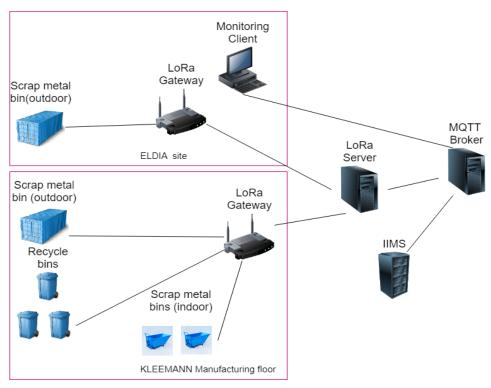
Figure 12 - UC-KLE-3 Sensors Network Architecture
