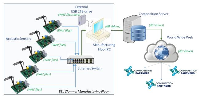
Figure 2 - Overview of the acoustic system
