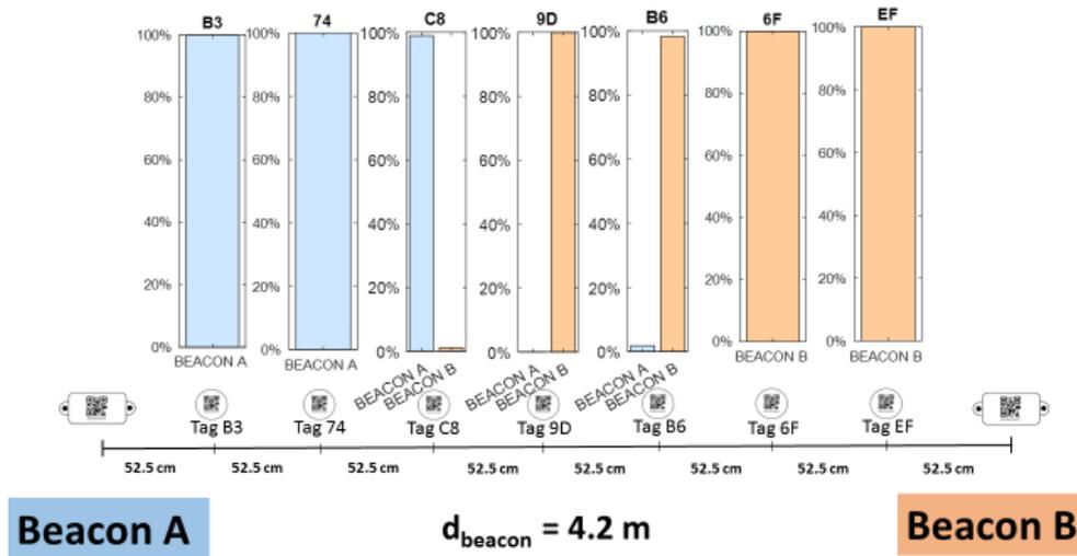
Figure 17. Test A – Regularly Spaced Tags Reported Positions Over 48 Hours
