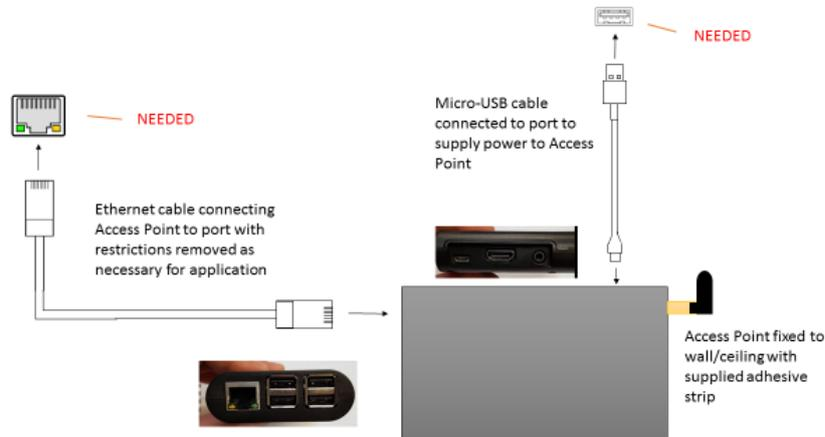
Figure 5. Access Point Required Setup
