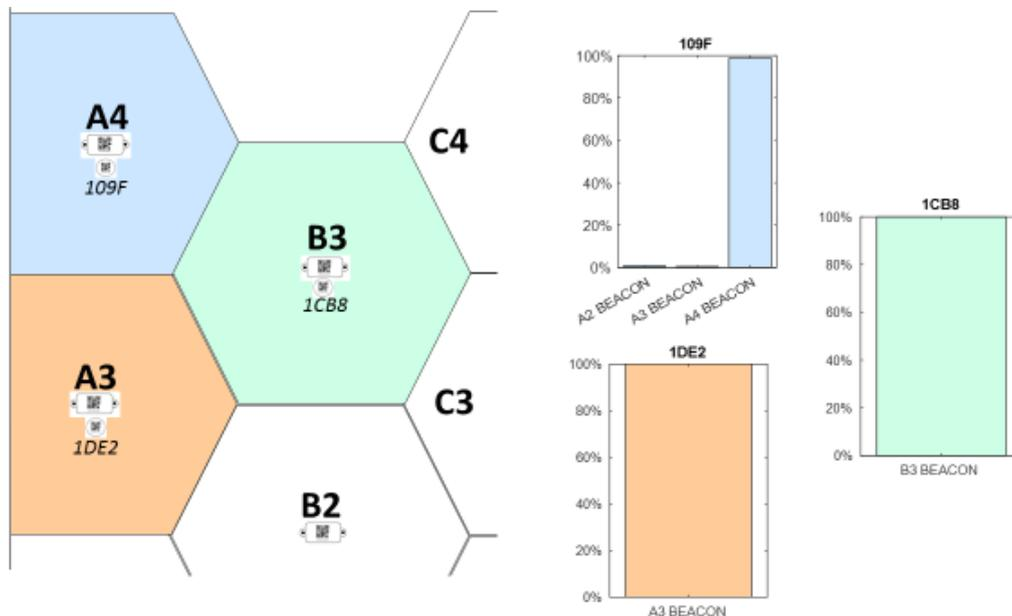
**Figure 19. Test C - Deployment Verification of Static Tracking (Reported Positions Over 48 Hours)**
