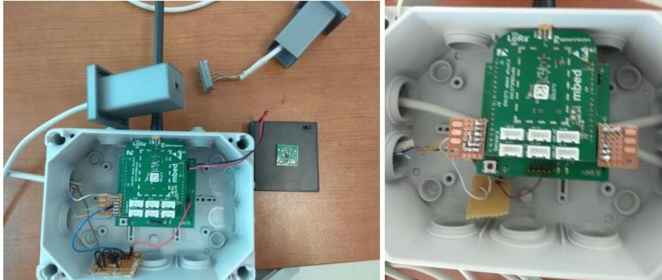
Figure 24: Fill Level Sensor for (a) Single (b) Multiple Bins
