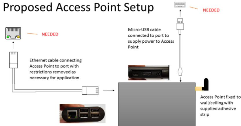
**Figure 7: Access Point Requirements**
