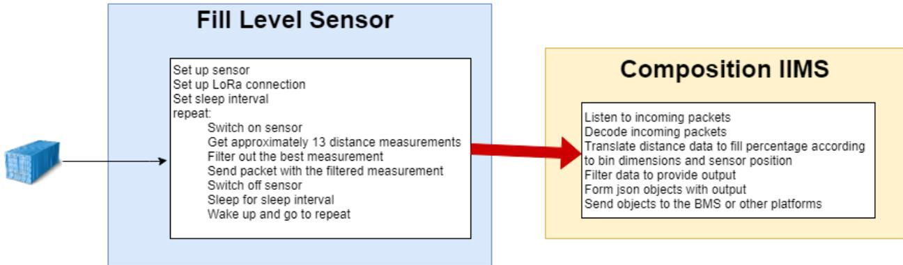
**Figure 20: UC-ELDIA-1 & UC-KLE-4 Software Architecture**
