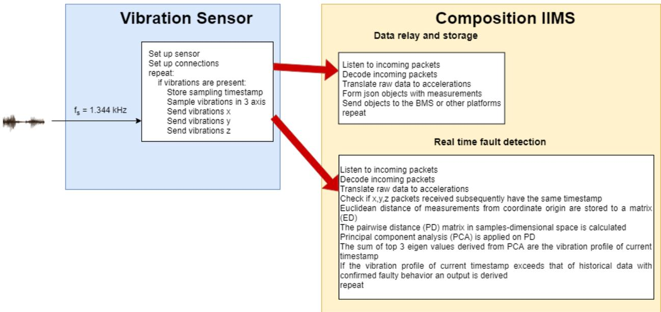
Figure 22: UC-KLE-6 Software Architecture
