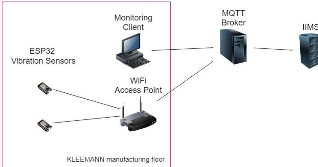
**Figure 21: UC-KLE-1 Predictive Maintenance Architecture**
