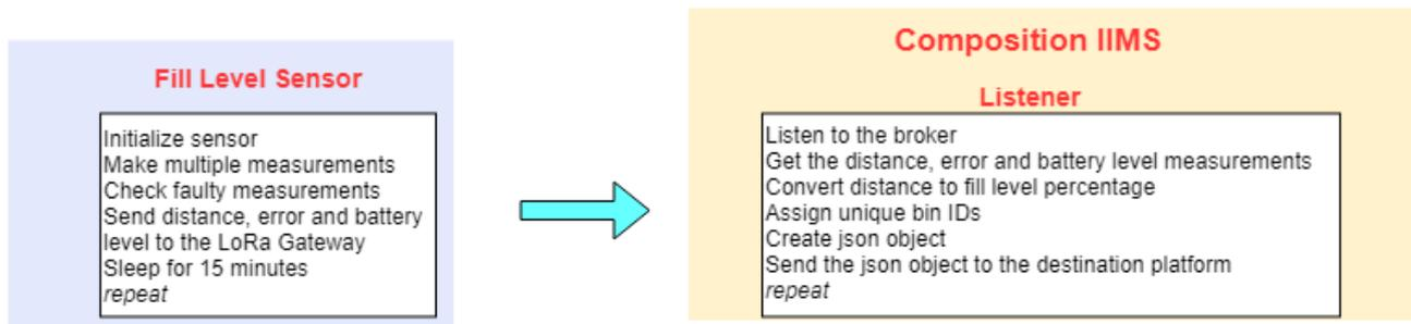
Figure 25: UC-KLE-3 Software Architecture
