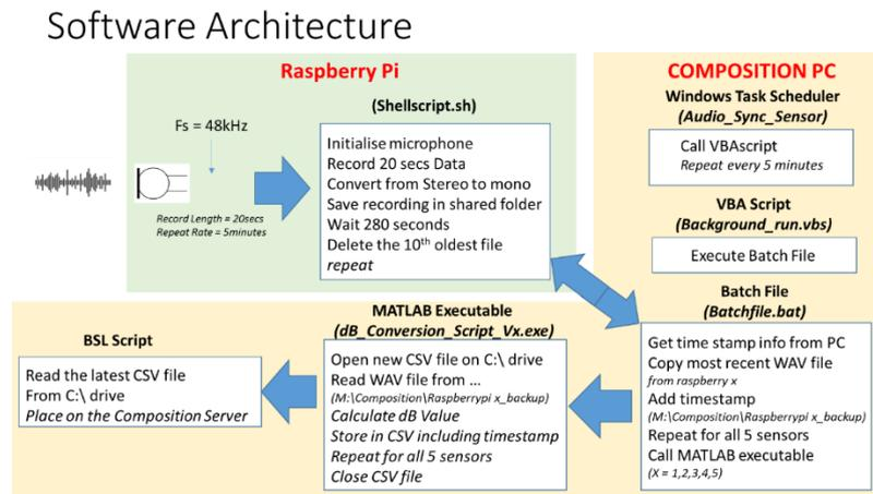
**Figure 2: UC-BSL-1 Software Architecture**
