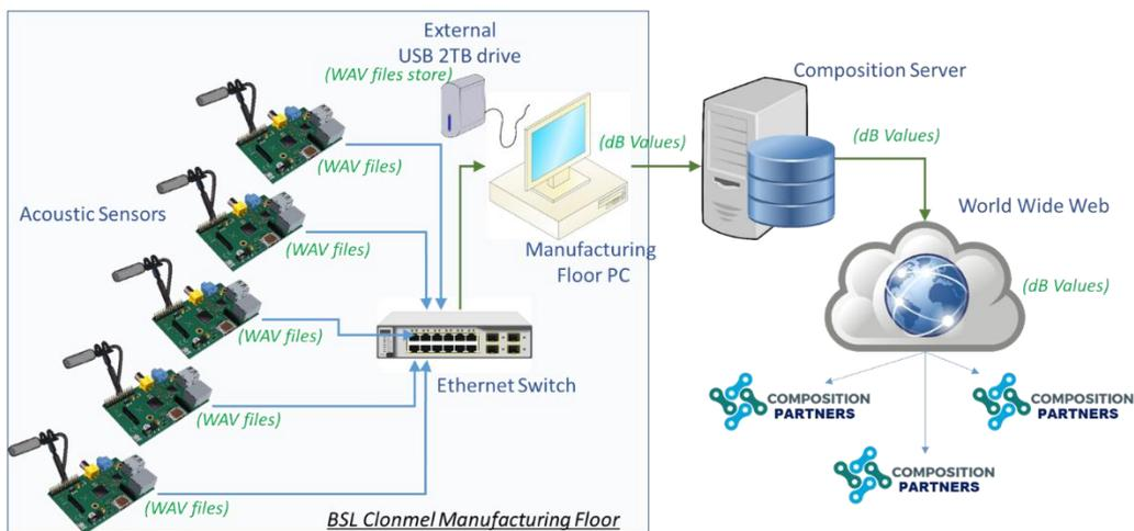
**Figure 1: UC-BSL-1 Condition Monitoring Architecture**
