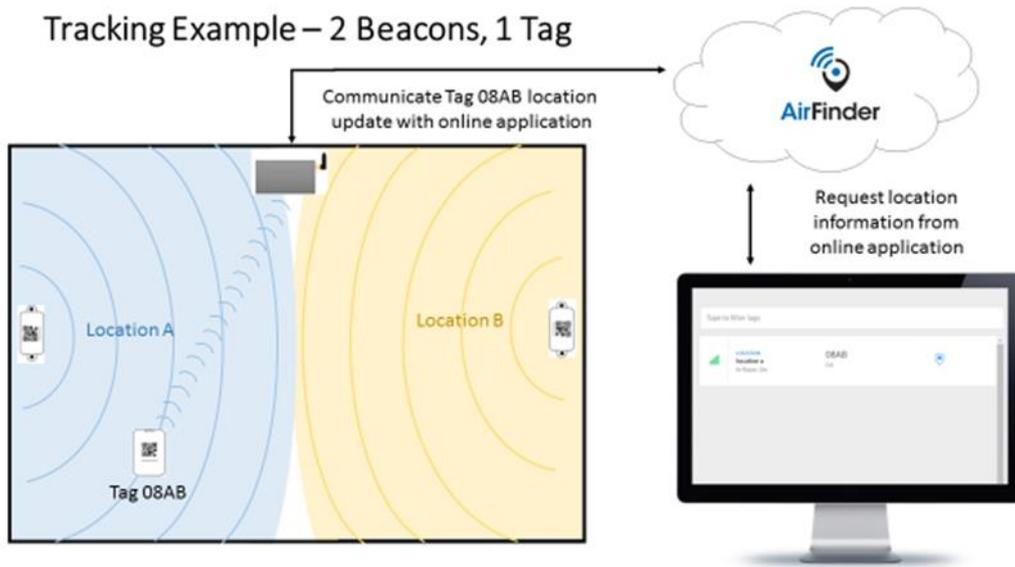
**Figure 3: Air Finder Configuration Tracking Example**
