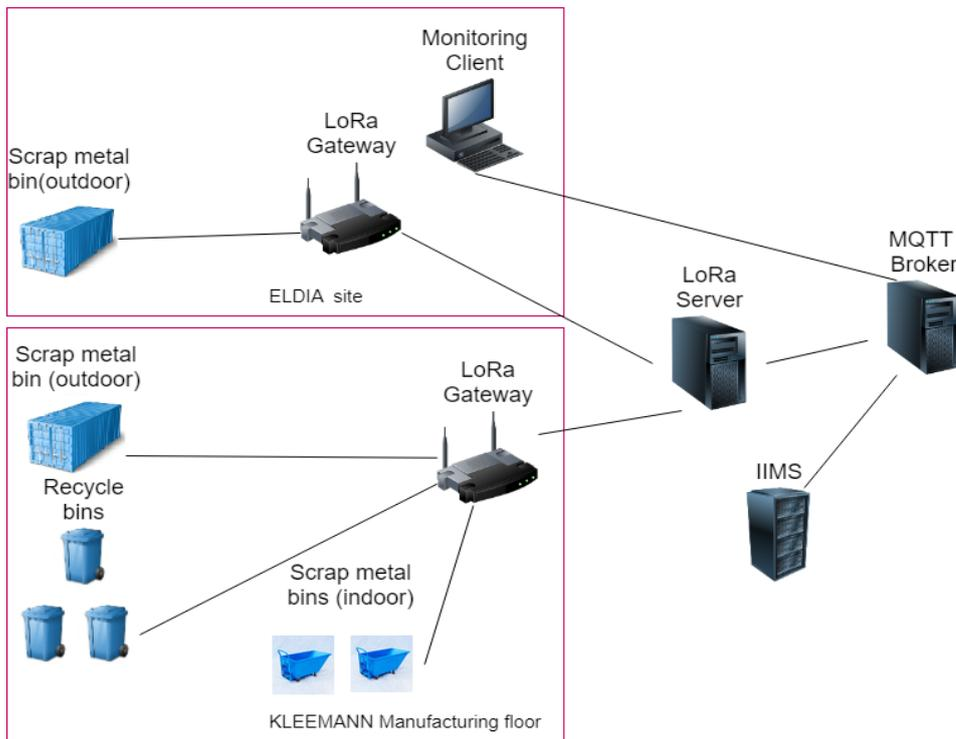
Figure 19: UC-ELDIA-1, UC-KLE-4 & UC-KLE 3 Architecture
