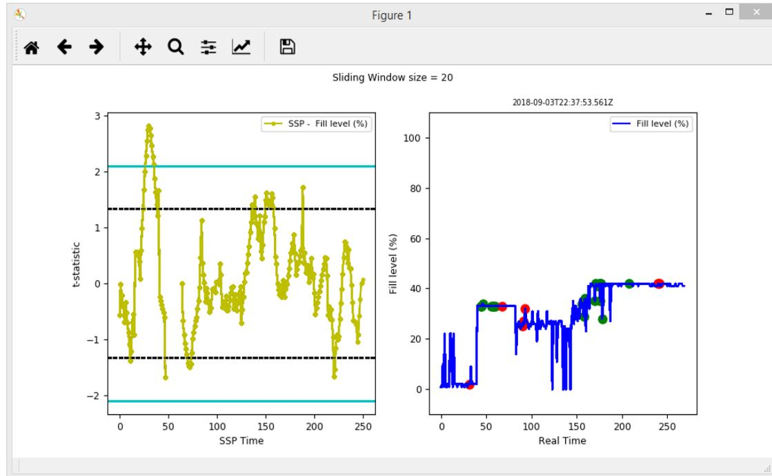
**Figure 7: Linear trend profile (left subplot) and fill level time series (right subplot) during the detection of changes in linear trend. The cyan and dotted lines in negative denote the Lower<sub>1</sub> and Lower<sub>2</sub> thresholds, respectively, and the cyan and dotted lines in positive denote the Upper<sub>1</sub> and Upper<sub>2</sub> thresholds, respectively.**
