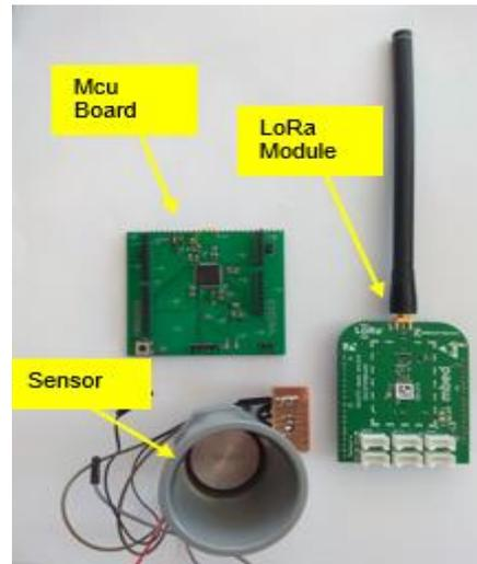
**Figure 3: Fill level sensor system overview**
