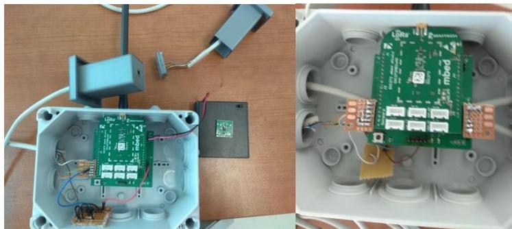
Figure 13: Fill level sensor for (a) single (b) multiple bins
