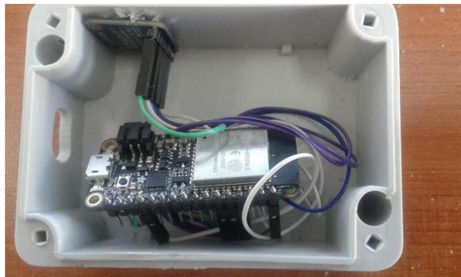
**Figure 10: Vibration Sensor**
