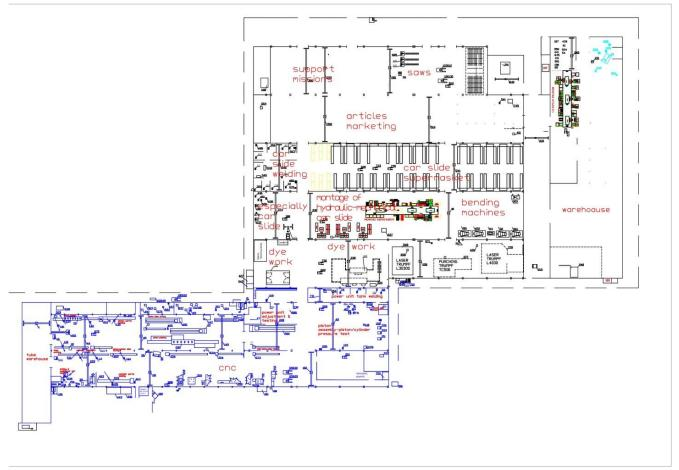
Figure 18. Floor plan of KLE manufacturing plant
