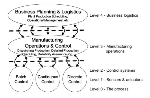
Figure 1. Layers of ISA95 Reference Architecture
