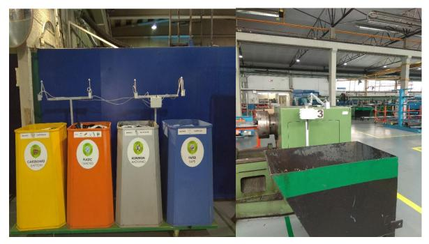
Figure 17. Images of recycling material containers (left) and scrap waste containers (right) and the installed fill level sensors in KLE
