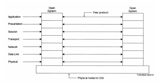
Figure 5. Layers of the OSI communication Model
