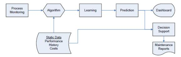
Figure 9. Diagram of proposed predictive maintenance process for BSL
