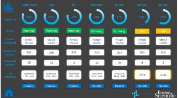
Figure 15. Concept of the line visualization screen
