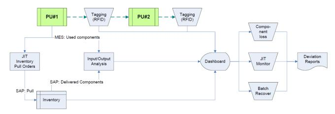
Figure 12: Diagram of proposed component tracking method in BSL
