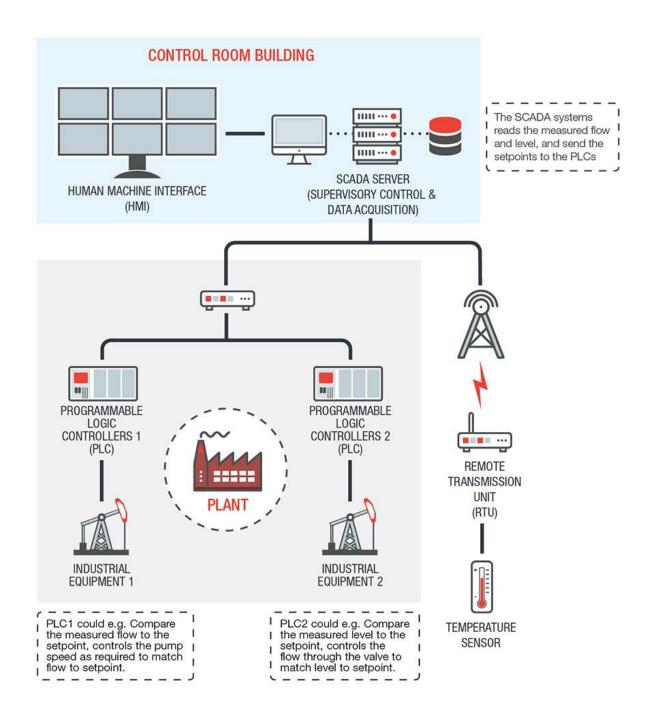
Figure 3 Example of a SCADA implementation
