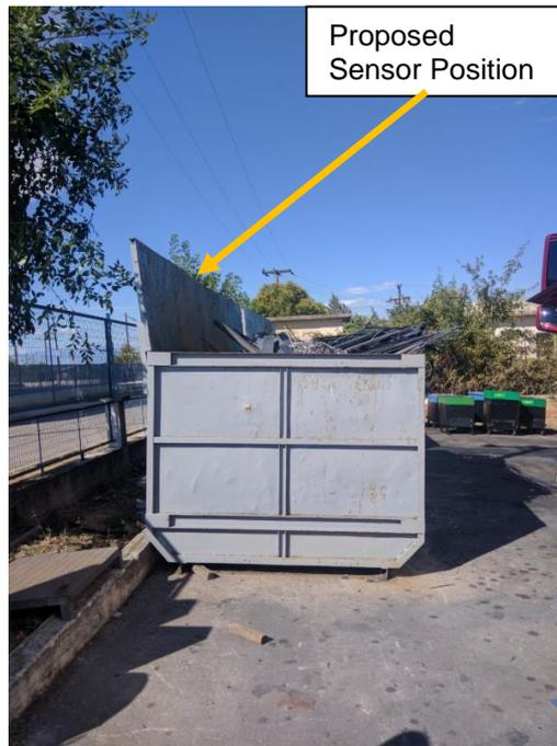
Figure 13: Proposed sensor position in scrap metal container
