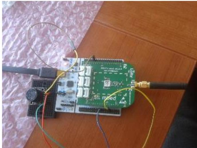
**Figure 19: Ultrasonic Sensor connected on STM32 Dev Board with Lora Communication Module**
