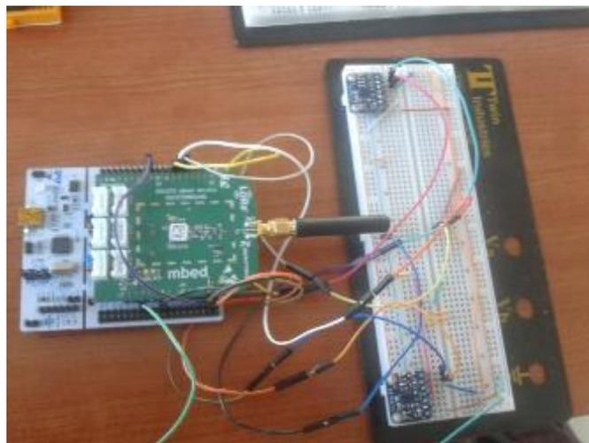
**Figure 20: A pair of VL53L0X sensors (Adafruit breakout boards) on STM32 Dev Board with Lora Communication Module**
