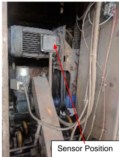
Figure 21: Bossi Motor (internal)
