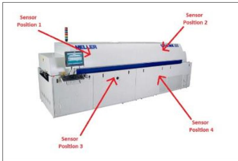
**Figure 9: Acoustic Sensor Placement for BSL**
