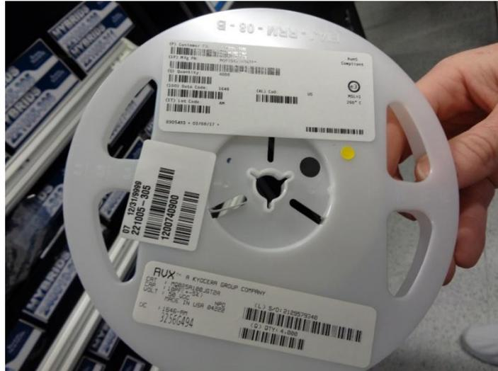
Figure 2. Example of a component reel
