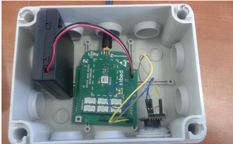
Figure 4: Fill level sensor system overview
