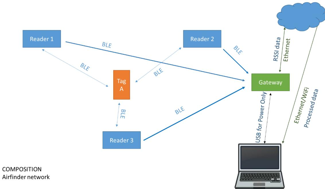
Figure 8 - Diagram of Airfinder’s information flow
