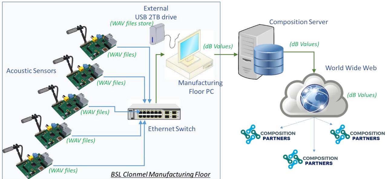
**Figure 2 - Overview of the acoustic system**
