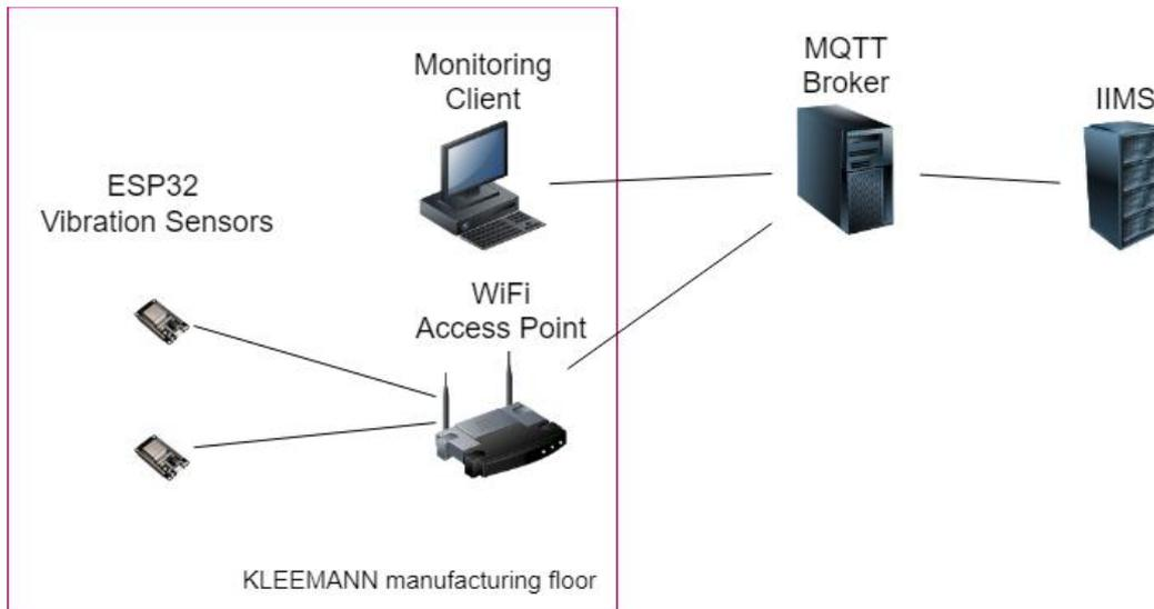
Figure 5 - UC-KLE-1 Sensors Network Architecture
