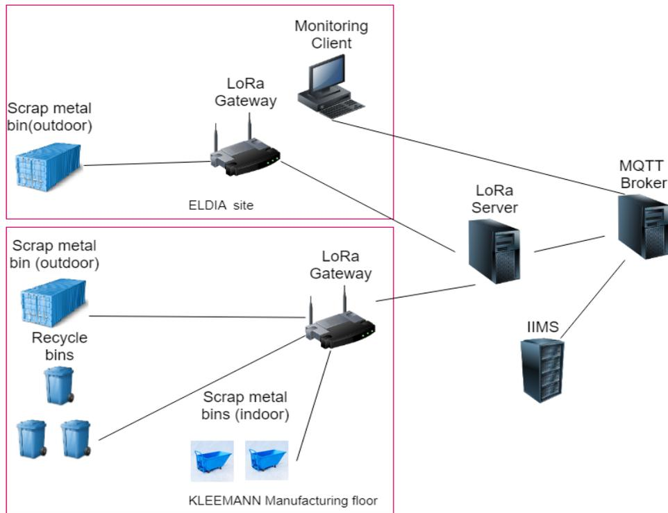
Figure 12 - UC-KLE-3 Sensors Network Architecture
