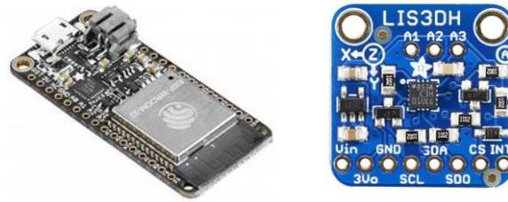
Figure 4 - ESP 32 board and Lis3DH on a Breakout Board
