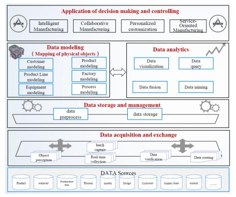
Figure 24: Industrial Internet Big Data Architecture Layers (source: Xiaohui, et al, 2018)
