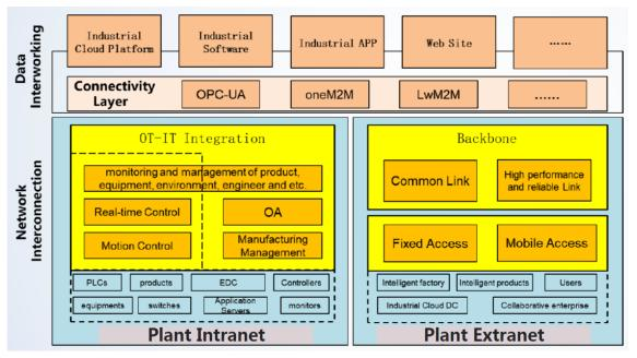
Figure 23: Connectivity Framework of Industrial Internet (source: Xiaohui, et al, 2018)
