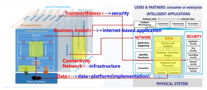
Figure 27: Convergence between IIRA and IIA (source: Xinhao Jiang, 2018)
