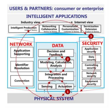
Figure 22: Industrial Value Chain Reference Architecture (source: Xiaohui, et al, 2018)
