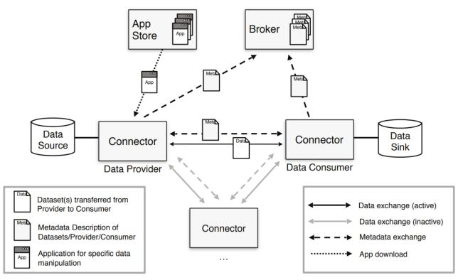
Figure 4: Interaction of components on System Layer (source: Otto, et al., 2019)
