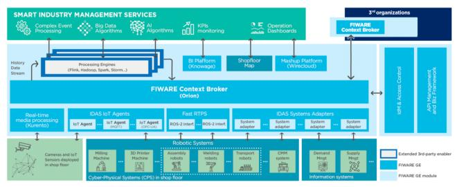
Figure 10: The FIWARE4Industry Reference Architecture (source: FIWARE, 2019)
