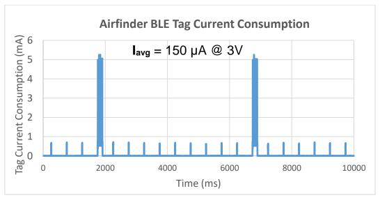
Figure 11. BLE Tag Current Consumption
