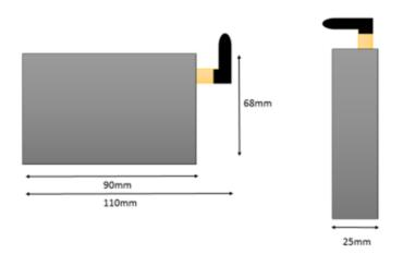
Figure 4. Access Point - Form & Dimensions
