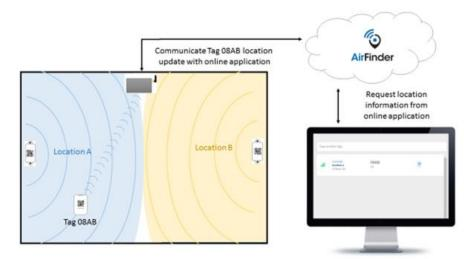
Figure 1. AirFinder Tracking Example (2 Beacons, 1 Tag)
