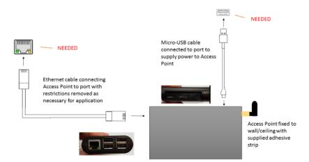
Figure 5. Access Point Required Setup
