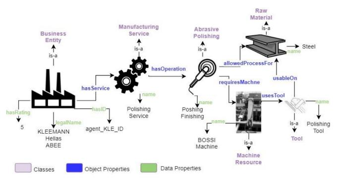
Figure 23: Modelling of KLEEMANN Polishing Procedure using Collaborative Manufacturing Services Ontology
