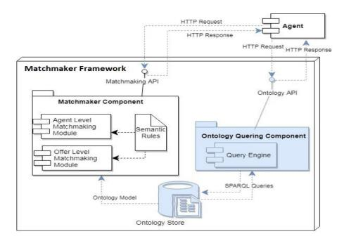
Figure 25: COMPOSITION Semantic Framework high-level architecture overview
