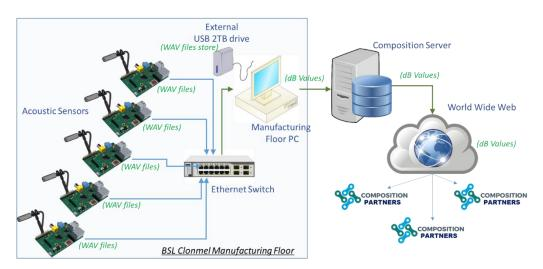
Figure 1: UC-BSL-1 Condition Monitoring Architecture
