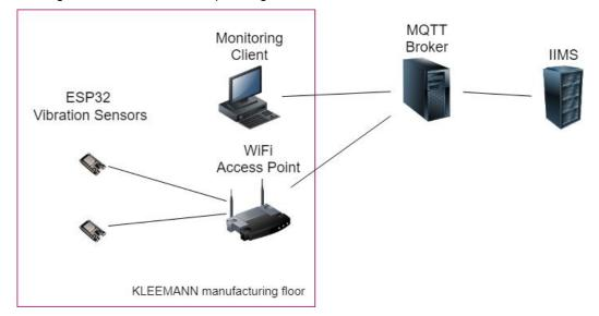
Figure 21: UC-KLE-1 Predictive Maintenance Architecture
