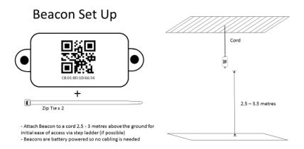
Figure 11: Beacon Set-Up
