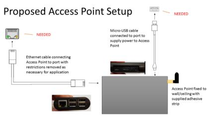
Figure 7: Access Point Requirements
