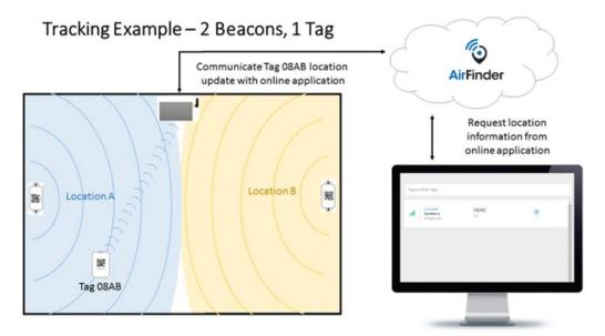
Figure 3: Air Finder Configuration Tracking Example
