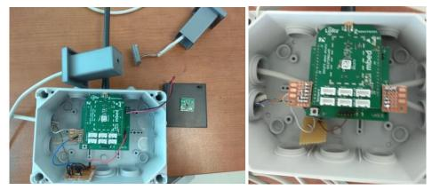
Figure 24: Fill Level Sensor for (a) Single (b) Multiple Bins
