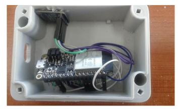
Figure 10: Vibration Sensor
