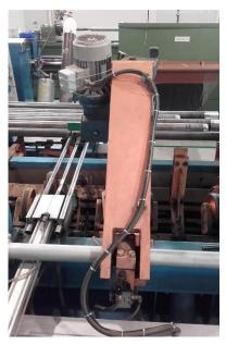
Figure 9: Vibration sensor position at Bossi machine
