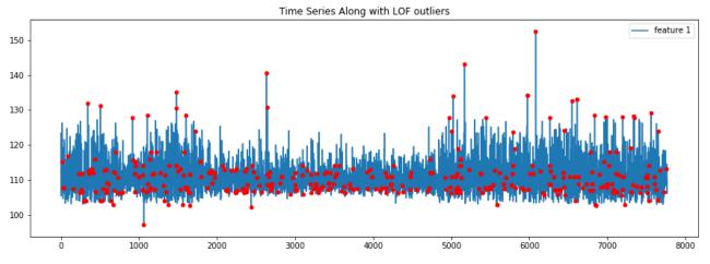
Figure 21: The LOF outliers pointed in the time series of the acoustic data of an indicative fan.
