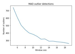
Figure 20: The ratio of number of detected outliers to the rolling window size.
