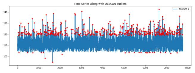
Figure 22: The DBSCAN outliers pointed in the time series of the acoustic data of an indicative fan.
