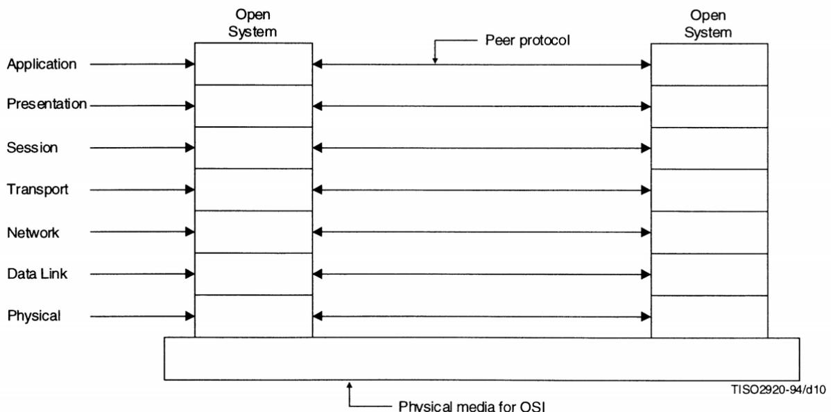
Figure 5. Layers of the OSI communication Model
