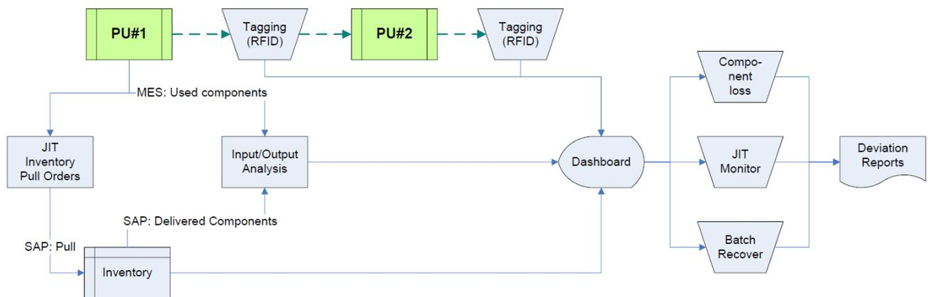
Figure 12: Diagram of proposed component tracking method in BSL
