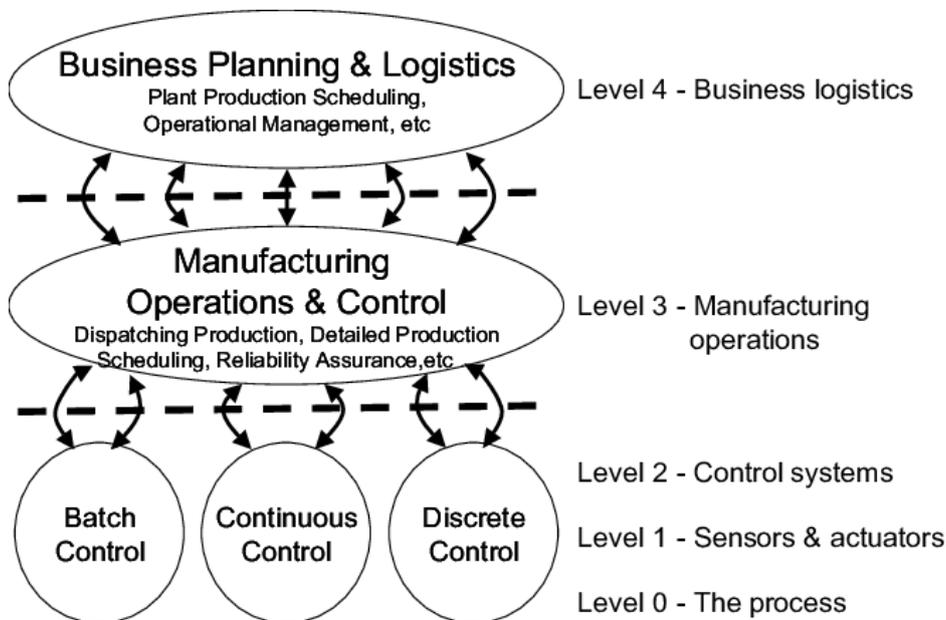
Figure 1. Layers of ISA95 Reference Architecture
