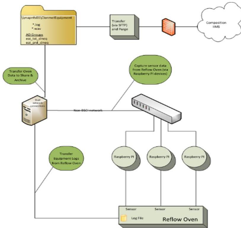
**Figure 11: Acoustic Sensor System diagram**
