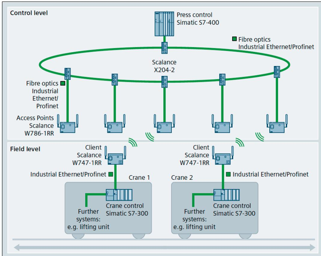
Figure 7. Commercial Example of a Communication Network
