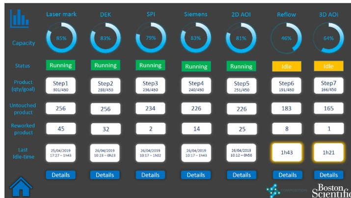
Figure 15. Concept of the line visualization screen
