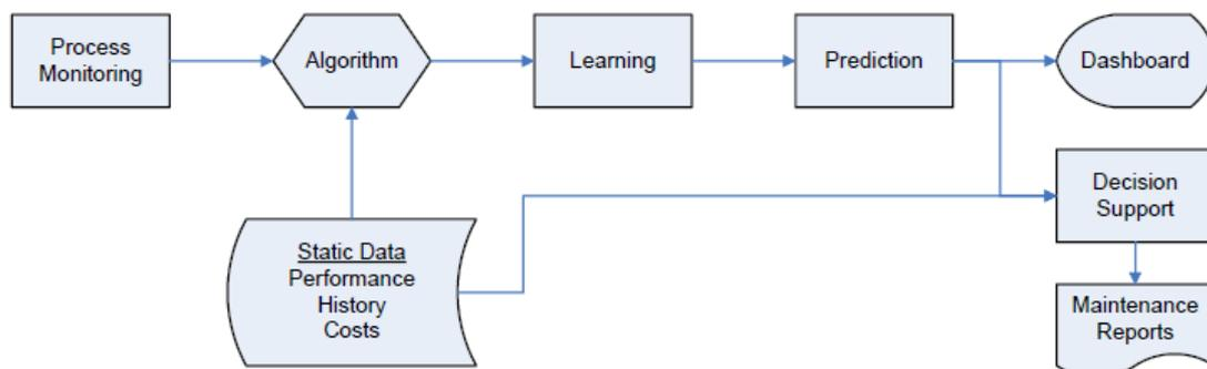
Figure 9. Diagram of proposed predictive maintenance process for BSL
