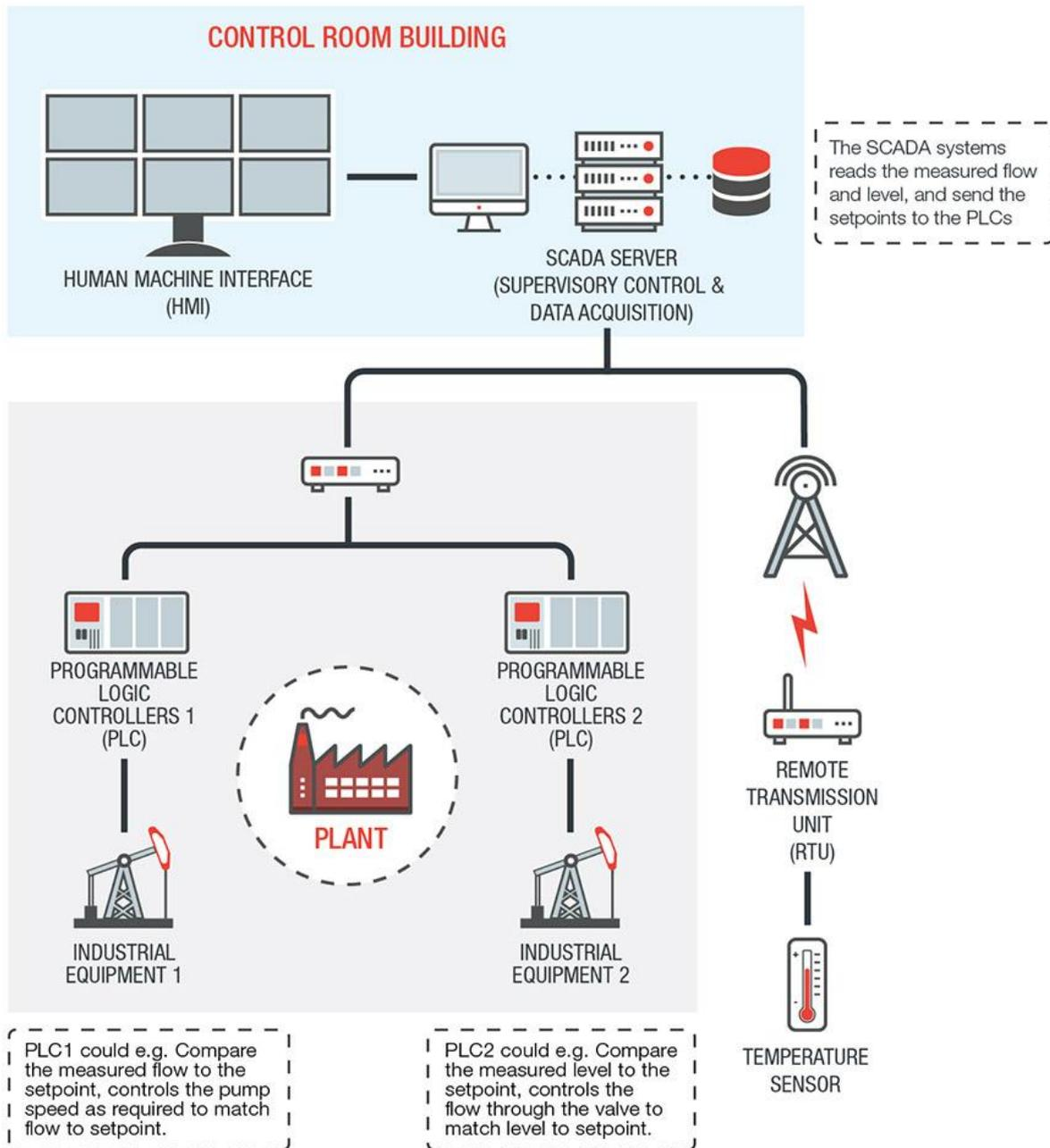
Figure 3 Example of a SCADA implementation
