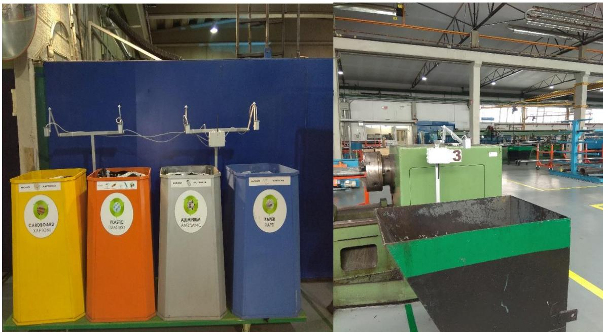
**Figure 17. Images of recycling material containers (left) and scrap waste containers (right) and the installed fill level sensors in KLE**
