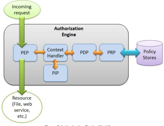
Figure 7 Authorization Engine Workflow
