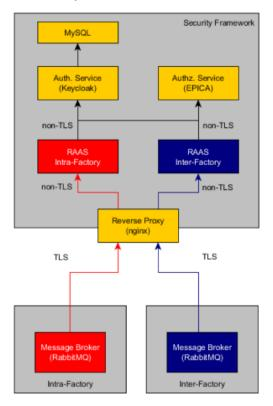
Figure 14 Security Framework architecture
