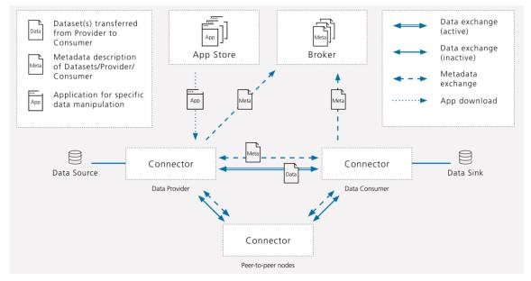
Figure 3. Interaction of components on System Layer (source: Otto, et al., 2018)
