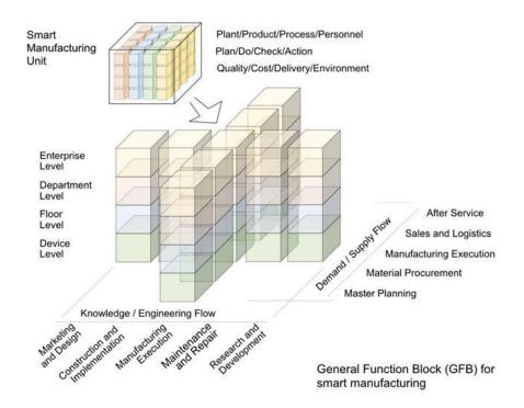
Figure 18 Industrial Value Chain Reference Architecture (source: Nishioka, Y., 2017)
