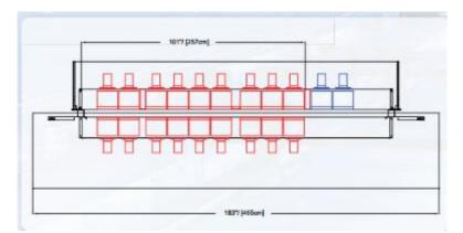
Figure 7: Layout of fans (blowers) in reflow oven
