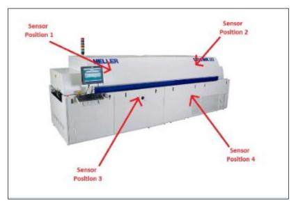
Figure 6: Position of sensors in BSL reflow oven
