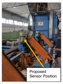
Figure 9: Proposed sensor position outside Bossi Motor
