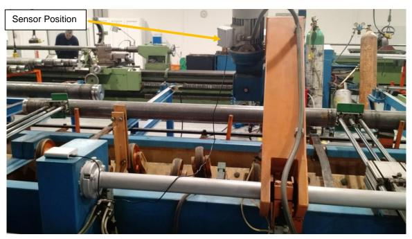
Figure 10: Actual sensor position outside Bossi Motor
