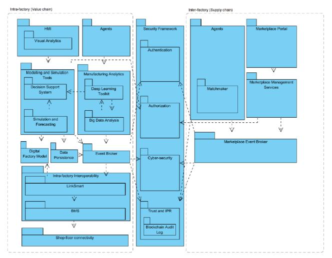
Figure 1: High-level functional view of COMPOSITION architecture.
