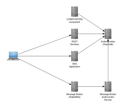
Figure 5: Possible interaction between Authentication and other components needing authentication
