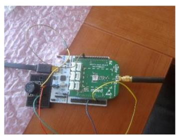
Figure 19: Ultrasonic Sensor connected onSTM32 Dev Board with Lora Communication Module
