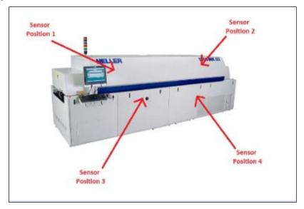
Figure 9: Acoustic Sensor Placement for BSL
