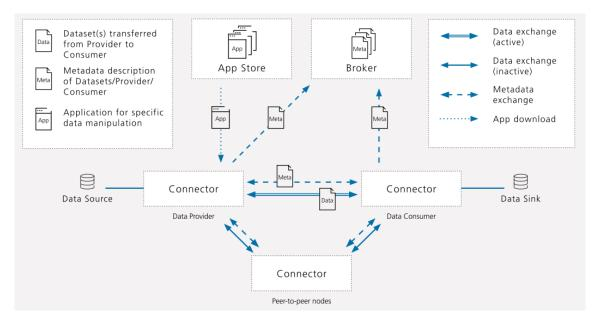
Figure 6. Interaction of components on System Layer (Otto, et al., 2017)
