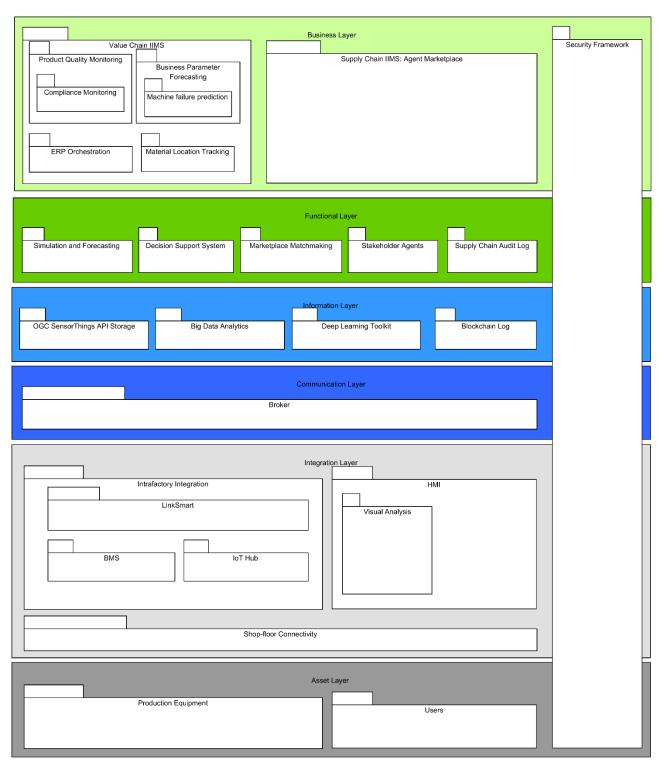
Figure 12. A mapping of COMPOSITION functional packages to the RAMI 4.0 Layers.
