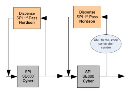
Figure 15. Proposed interoperability solution for autonomous solder paste dispensing in BSL
