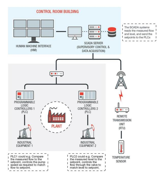
Figure 3 Example of a SCADA implementation
