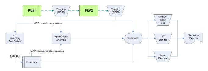
Figure 11. Diagram of proposed component tracking method in BSL
