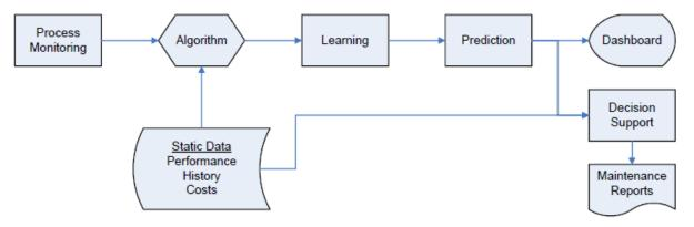
Figure 9. Diagram of proposed predictive maintenance process for BSL
