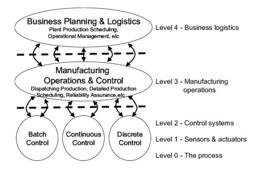
Figure 1. Layers of ISA95 Reference Architecture
