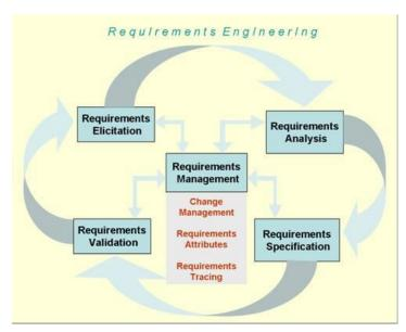
Figure 1: The Requirements engineering process
